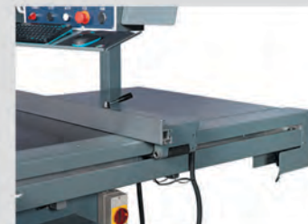
Servo driven motorized rip-fence Guarantees precise adjustment with high accuracy
