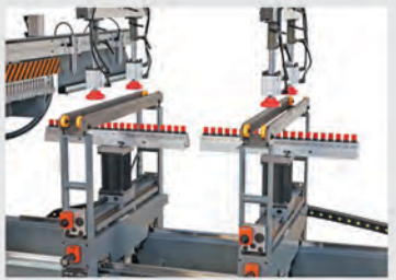
Vertical boring units can be turned 90°. Auxiliary support frame with fence gives better solution for long panels.
