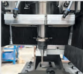
Patented : Upper spindle equipped with saw blade for horizontal slot
