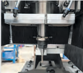
Patented : Upper spindle equipped with saw blade for horizontal slot
