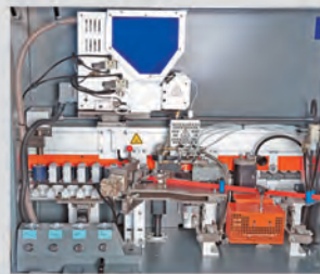
Top Glue Tank With Quick Melting Device Along With Bottom Glue Tank
