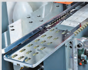
In-feed Plate with Roller for Easy Feeding
