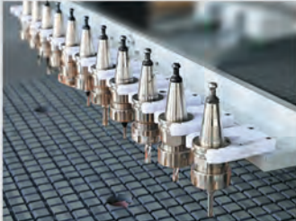
Linear type 12 auto tool changer on gantry to reduce time
