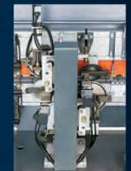
Servo Controlled Edge Scraping
