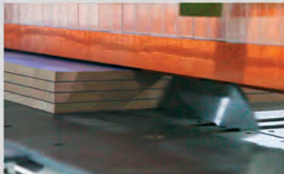
Maximum cutting thickness up to 100 mm.
