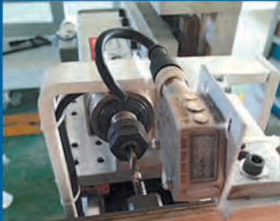
Air cooled 2.2 kw spindle with laser sensor & servo motor
