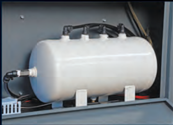
Safety Air Tank for Non-Dropping of Air During Process
