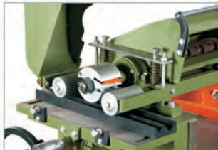
Auto Mould for straight moulding work
