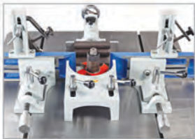
Fence for the setting of precise depth of cut. Fences can also be adjusted endwise.
